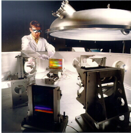
FIGURE 2.1: Photograph of the compressor under vacuum of the UHI10 CPA-based laser system (from http://iramis.cea.fr/femto/slic/index.php ).
